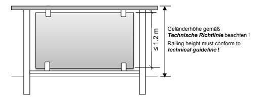
6.3 Balustrade with horizontal bars (protection against falling is provided solely by sufficiently strong handrails and knee-height bars)
