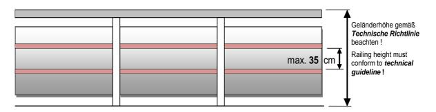
The type of glass used shall be selected from Table A, glazing not intended to protect against falls. The spacing between horizontal bars should not exceed approx. 35 cm.
